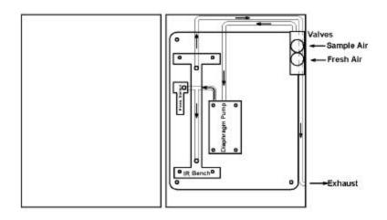
Figure 2 Pneumatics Diagram
